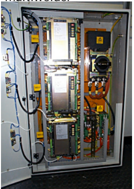
3 timers + 3 SCRs multiwelder
